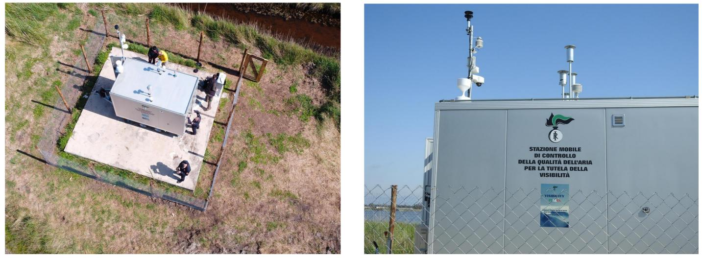
Fig. 2 The Visibility cabinet near the Lago dei Monaci, drone view and focus on the sampling lines for particulate matter and the meteorological measurements
