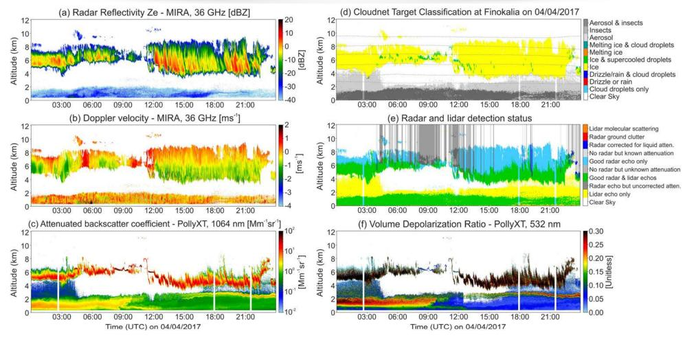
Radar reflectivity (a), radar Doppler velocity (b), and lidar attenuated backscatter coefficient (c) measured on 4 April 2017 in Finokalia, Crete. Cloudnet target classification (d), radar/lidar detection status (e), and lidar volume depolarization ratio (f) for the same day (Marinou et al., 2021).
